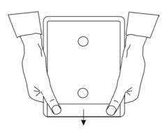
The terminal cap will then spring out of the two detent clips.
