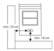
Installing the Gigaset HC450 door intercom system
