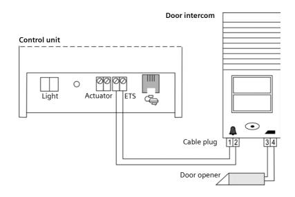
Installing the Gigaset HC450 door intercom system
