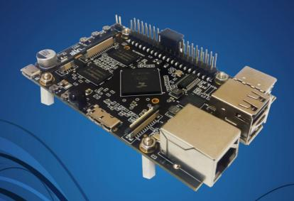
Quad-core Cortex-A9 ARM processor
