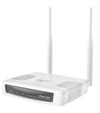
The ALLNET ALL02850N is a Wireless N300 Indoor Access Point with 29 dBm transmit power for long range coverage, wireless speeds up to 300 Mbps and a Fast Ethernet port for connecting to a switch or router. With its enhanced receive sensitivity and its MIMO (Multiple In/Multiple Out) antenna array extends wireless coverage and enhances connectivity to client devices.
